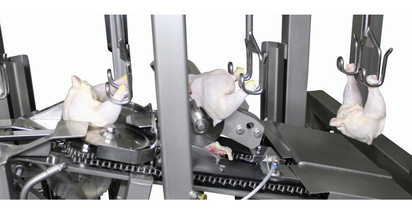
The Foodmate Breast Processor runs birds breast first. An arbour and several guidings pick up the bird and guide them into the circular blade. The breasts are then cut and transported through the machine by the pick-up chains.
