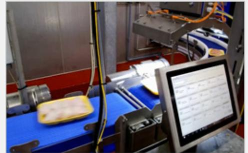
Utilising inVISION Camera Grading System from Foodmate, the system can recognise and sort products according to customer requirements.
